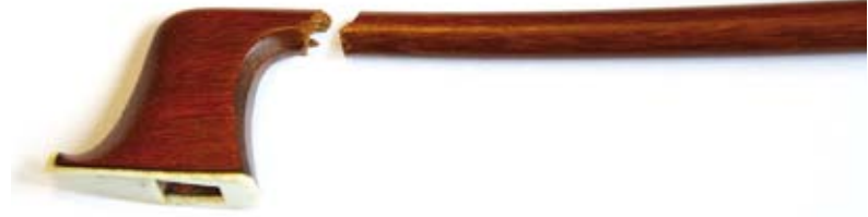
Fatigue fracture of a wooden bow
